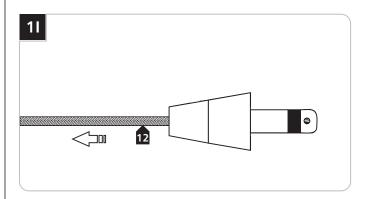
Pull the coaxial cable toward the fixture to smooth the wrinkles.
