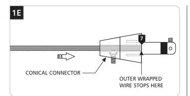
Feed and push the coaxial cable into the conical connector. The coaxial cable will come to a stop point after being inserted 3/4" into the conical connector.
