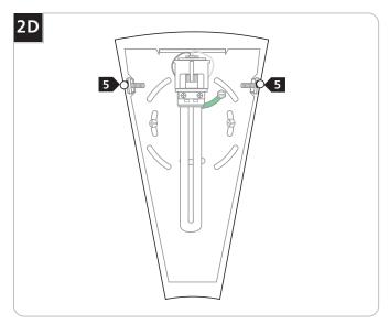
Firmly push the glass against the wall and finish tightening the ball screws.
