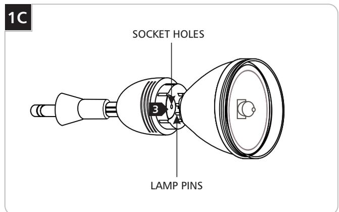
**3** Line up the lamp pins with the socket holes. Insert the MR16 lamp pins into the socket holes, simultaneously push the accessory shade onto the grooved shade holder.
