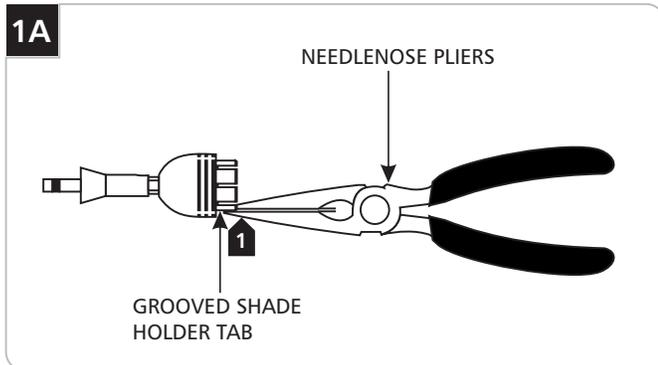
**1** If the accessory shade fits tight or loose onto the Tilt fixture, then carefully bend the grooved shade holder tabs in or out slightly with needle-nose pliers.
