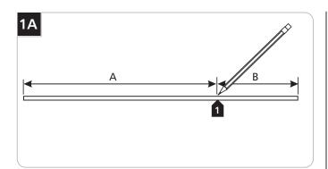
1 From one end mark the section of the extender that needs to be shortened (B), refer to the chart below for measurements.
