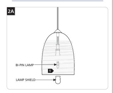
**1** Remove the lamp shield and the old lamp.
