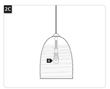
4 Push the lamp shield onto the spring clip.
