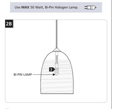
2 Handle the new replacement lamp with a soft cloth to prevent the natural oils on the fingertips from collecting on the lamp. This will help extend the life of the lamp.
