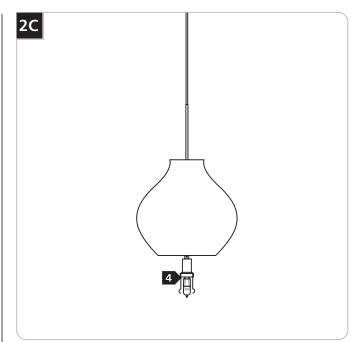
Use MAX 50 Watt, Bi-Pin Halogen Lamp.
