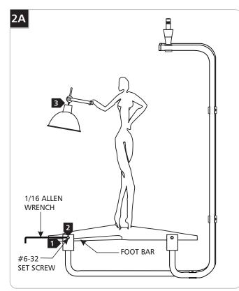
Insert each end of the foot bar all the way into one connector slot.
