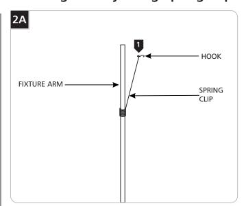
**NOTE:** Use this installation only when bare (uninsulated) Kable Lite cables are used.
