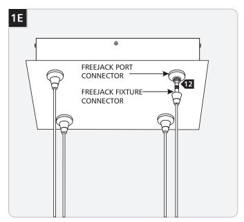
Screw the FreeJack fixture connector to the FreeJack port connector.
