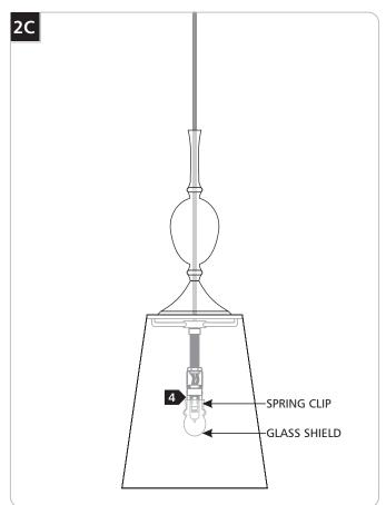
4 Push the lamp shield onto the spring clip.
