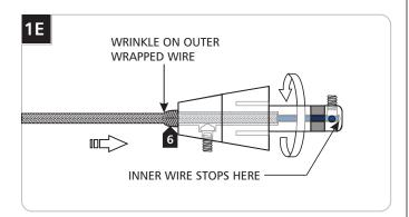
6 Keep pushing the coaxial cable into the connector while rotating the connector to ease feeding the inner wire into the tip of the connector. The outer wrapped wire will start wrinkling while being inserted another 1/2" into the connector.
