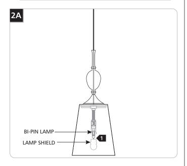
Use MAX 50 Watt, Bi-Pin Halogen Lamp.
