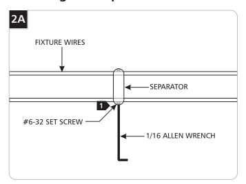
**NOTE:** To avoid an electrical short between the fixture wires, a separator must be snapped between the fixture wires so that the wires are equal distance from each other.
