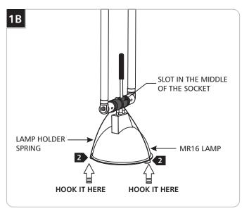
2 Hook one end of the lamp holder spring (provided with the package) onto front of the lamp. Wrap the spring over the slot in the middle of the socket and hook the other end onto front of the lamp.
