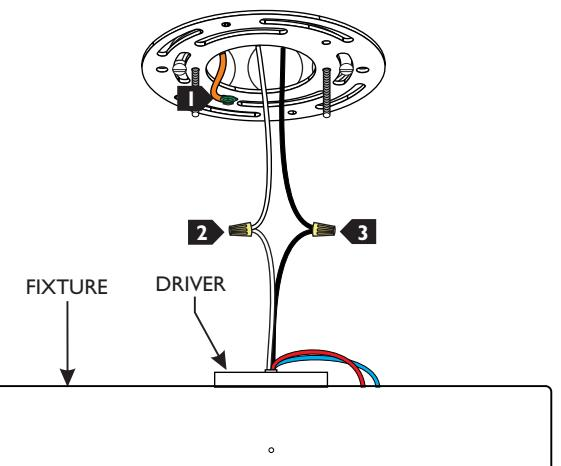
**1** Connect the mounting plate ground wire to a suitable ground in accordance with local electrical codes.
