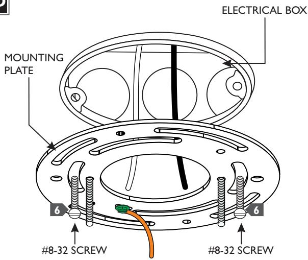
**6** Mount the mounting plate to the electrical box with the two #8-32 screws.
