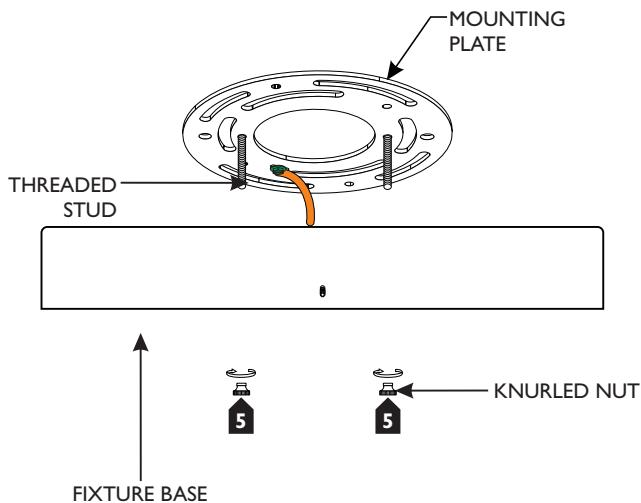
**5** Remove the mounting plate from the fixture base by unscrewing the two knurled nuts from the two threaded studs.
