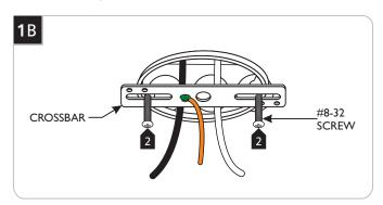
2 Mount the crossbar assembly to the electrical box with the two provided #8-32 screws.
