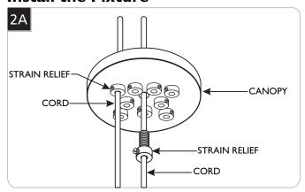
1 Feed a fixture cord through each the strain relief.
