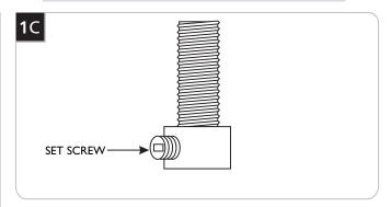
Loosen (**Do Not Remove**) the set screw on each strain relief.
