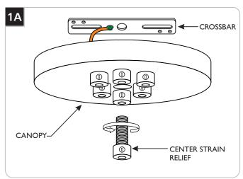
1 Remove the crossbar from the canopy by completely unscrewing the center strain relief.
