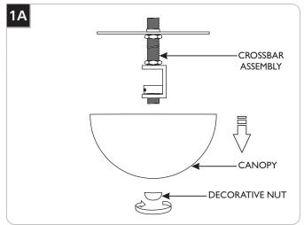
1 Separate the crossbar assembly from the canopy by unscrewing the decorative nut from the crossbar assembly.
