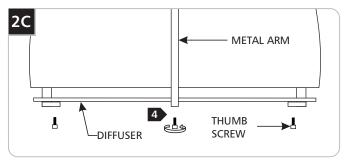
4 Screw a thumb screw through each metal arm and into each threaded hole in the diffuser.
