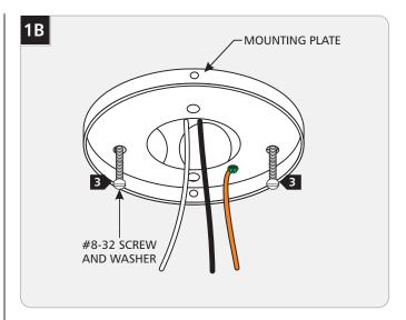
Secure the mounting plate to the electrical box with the two washers and #8-32 screws provided.
