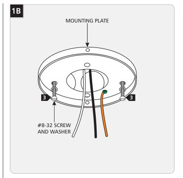
Secure the mounting plate to the electrical box with the two washers and #8-32 screws provided.
