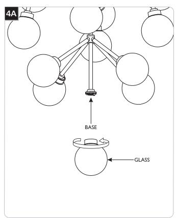
1 Install the glass by screwing it into the base. **Do not over-tighten.**
