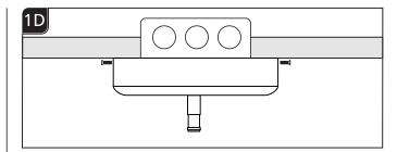
Reattach the transformer to the mounting plate by securing it with the two screws.
