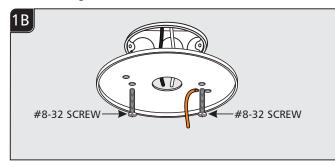
Attach the mounting plate to the electrical box using the two #8-32 screws provided.
