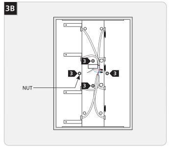
Mount the pan to the backplate with the provided washers, lock washers, and nuts.
