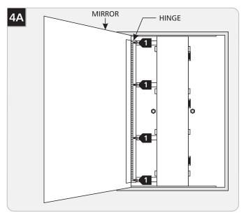
1 Carefully attach the mirror hinge onto the fixture and tighten all four screws.
