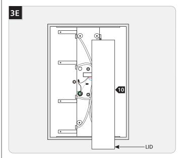
10 Replace the lid onto the center of the housing and tighten the screws.
