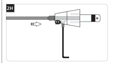
Firmly tighten the set screw on the conical connector.
