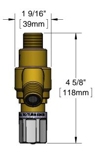
Water from Exceeding Customer's Maximum Temperature Set Point. Valve is Factory Pre-set to Deliver Mixed Water Temperature of Approximately 100°F (38°C) Max.
