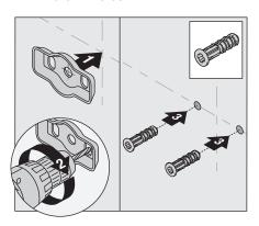
2b) **Stud Option:** Place mountin brackets into desired position. Using brackets as a guide, carefully drill 1/8" holes into wall.
