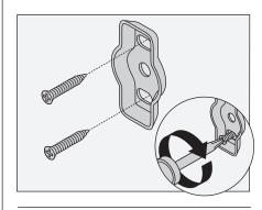
8) Hang top of accessory on mounting bracket. Lower into position
