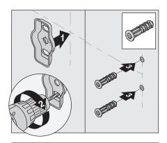
6b) **Stud Option:** Place mounting brackets into desired position. Using brackets as a guide, carefully drill 1/8" holes into wall.
