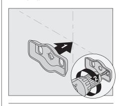
With mounting brackets in position, secure to wall using screws.
