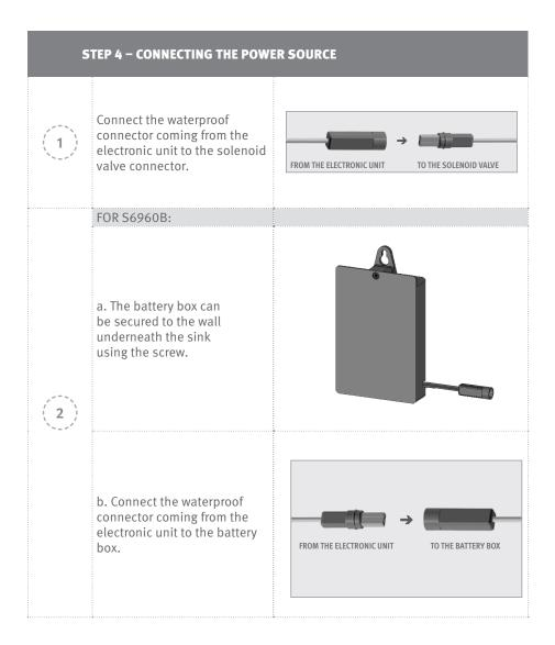
a. Connect the waterproof connector coming from the electronic unit to the
