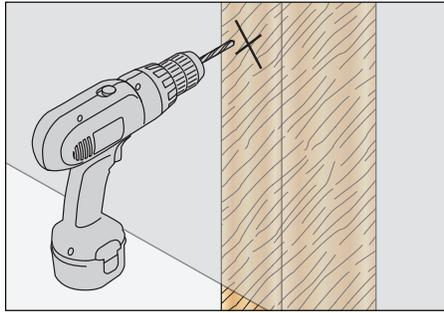
2) Remove Toilet Paper Holder from wall. Use drill with 7/64" drill bit to drill holes into wall and wall studs at the marked positions.
