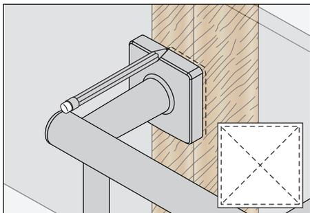
1) Place Toilet Paper Holder at desired position. Mark the centers on each end with a pencil. Follow steps 1-3 for wall and wall studs (page 3) to install bracket to wall stud.
