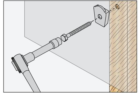
3) Use ratchet and lag bolt to attach mounting bracket to wall. Do not overtighten. Repeat step for opposite end, and then tighten both brackets so they are secured to wall.
