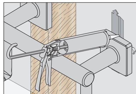
9) Apply a bead of silicone around the perimeter of the Toilet Paper Holder ends to prevent water from bleeding through the mounting holes and potentially damaging the wall and wall studs.
