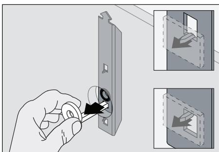
4) Pull backward on white flange so bar straightens and tilts upright. Arrow on bar must be facing upwards for anchor to perform as intended.
