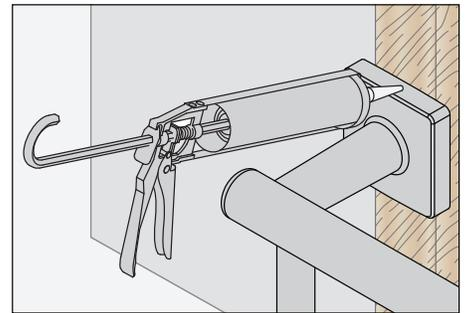
6) Apply a bead of silicone around the perimeter of the Toilet Paper Holder ends to prevent water from bleeding through the mounting holes and potentially damaging the wall and wall studs.
