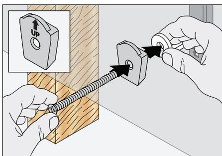
5) Keep pressure on bar behind the drywall. Align holes in bar, white flange and bracket. Align machine screw with holes. Hand tighten machine screw so bar remains upright.
