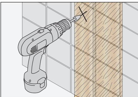
1) Follow step 1 for wall and wall studs to mark centers of Toilet Paper Holder ends. Use drill with 5/16" carbide tip drill bit to drill holes into ceramic tile at the marked positions to prevent damage to the tiles.
