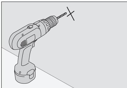
2) Use drill with 1" drill bit to drill holes into drywall at the marked position.
