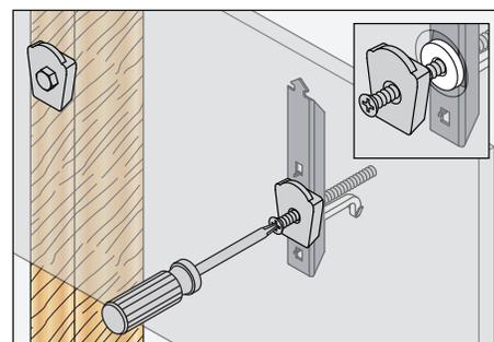
6) Tighten machine screw with phillips head screwdriver so bracket attached to mounting anchor bar is flush with drywall.
