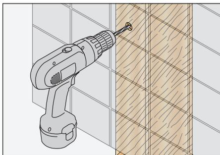
2) Use drill with 7/64" drill bit to drill pilot holes into wall studs through ceramic tile.
