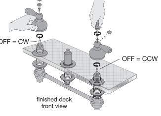
Step 6 Fasten valve assembly to deck
