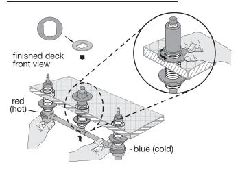
Step 4 Attach valve assembly
