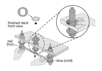
Step 4 Attach valve assembly to deck
