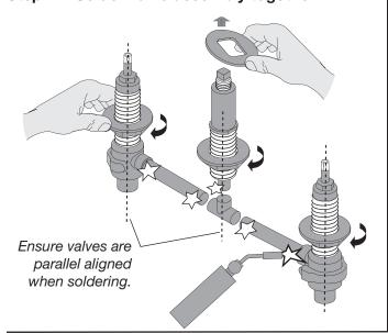
Step 3 Mount valve assembly to deck
