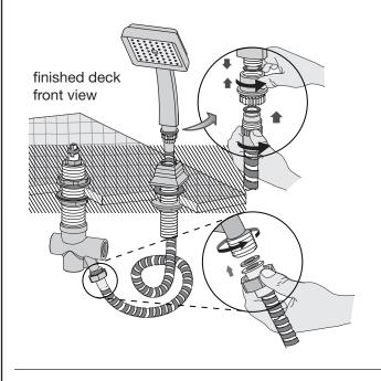
Step 7 Install plping and check for leaks
