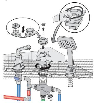
Step 11 Flush supply lines; check for leaks
