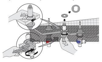
Step 3 Install diverter valve adapters (3)
