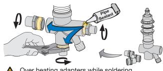
Over heating adapters while soldering can damage thread seal. Ref. Step 7
