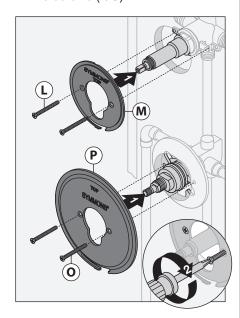
2) Attach diverter escutcheon (K) to small mounting plate (M).
