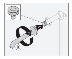
10) Install showerhead (D) to shower arm (B). Turn clockwise to tighten.
