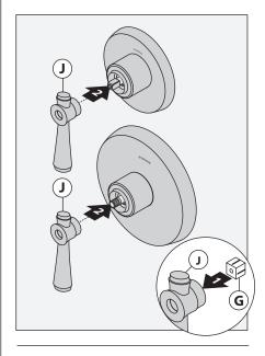
6) Secure handle(s) to valves using star washer (F) and screw (I).
