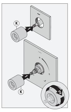
5) Install diverter handle (J) and shower handle (J) to valves. Secure handles by tightening set screws.
