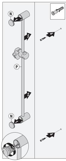
**Notes:** Make sure that slide bar holes and bracket holes are aligned before drilling. Before drilling bottom hole, make sure slide bar is plumb.
