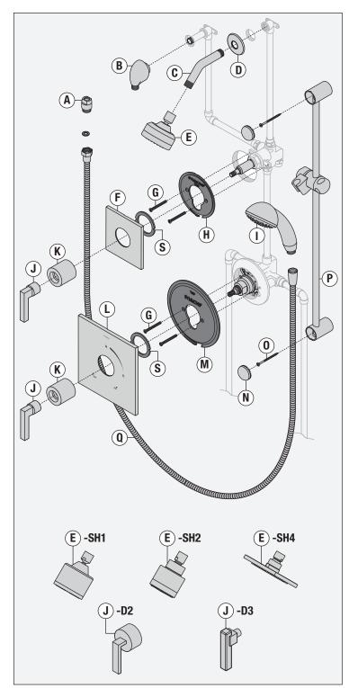
Notes: 1) Apply a bead of silicone around the perimeter of all shower trim installed flush to the finished wall. Leave opening on bottom of escutcheon for weep hole.2) Apply plumber tape to all threaded connections.
