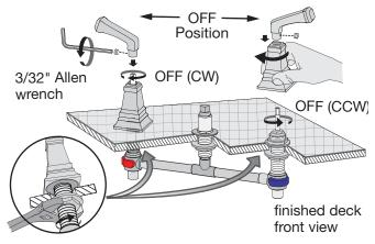
Step 6 Solder supply lines to valve inlets and check for any leaks
