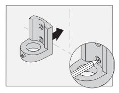
2a) **Dry Wall Option:** Carefully drill 3/16" holes into wall. Install anchors into holes.
