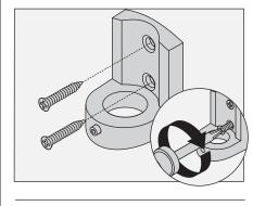
Insert rod brackets into mounting brackets and secure with Allen screws.
