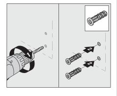
2b) **Stud Option:** Carefully drill 3/16" holes through wall and into studs.
