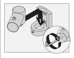
5) Insert shower rod into rod brackets and secure with Allen screws.
