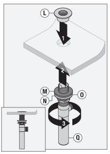
**Note:** Make sure drain cavity (on drain body) faces rear of sink.
