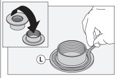
5) Insert flange (L) into drain opening. From below, attach drain body (Q) with washers (M, N, and O) to flange (2-3 turns until hand tight).
