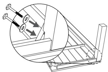
Insert the bolt through a washer from the corner-block onto the leg. Tighten it firmly with 12mm(1/2') wrench.
