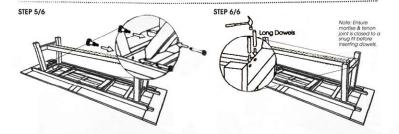
Insert and tighten 2 Bolts into the pre-drilled holes on the leg support, as shown ine picture. Repeat step for the other side,
