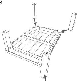
Insert the bolt through a washer from the corner-block onto the leg. Tighten it firmly with 12mm (1/2') wrench provided.
