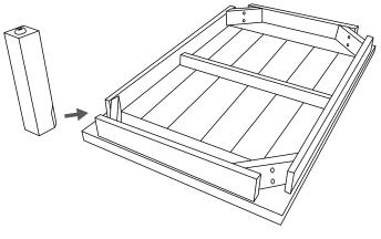
Lay Top section flat on level surface. Bottom side facing upward.
