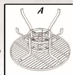
.) Begin to gently tighten all nuts or bolts in succession, never torque ne bolt completely as this could make the table wobble. Instead, tighten ach bolt slightly, then move to the next in succession until all bolts are ecurely fastened.
