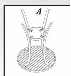
.) Begin to gently tighten all nuts or bolts in succession, never torque ne bolt completely as this could make the table wobble. Instead, tighten ach bolt slightly, then move to the next in succession until all bolts are ecurely fastened.
