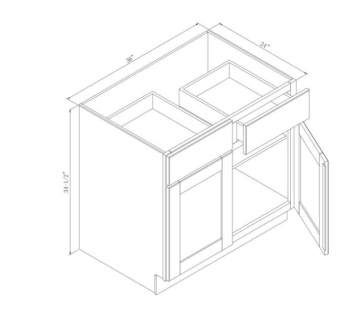
NOTE: No center stile. Batten is attached to door panel in lieu of a center stile.
