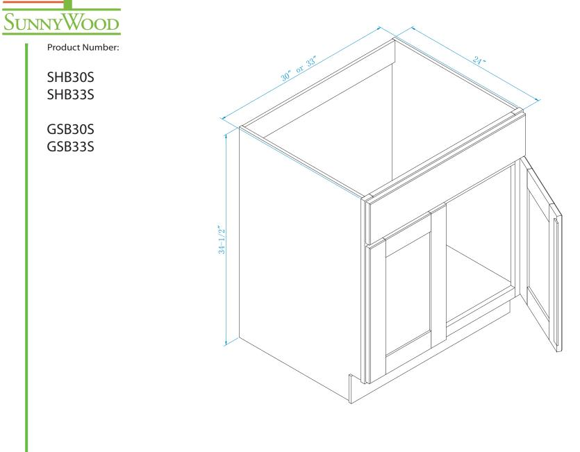
NOTE: No center stile. Batten is attached to door panel in lieu of a center stile.
