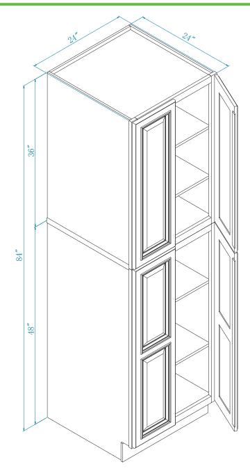
NOTE: No center stile. Batten is attached to door panel in lieu of a center stile.
