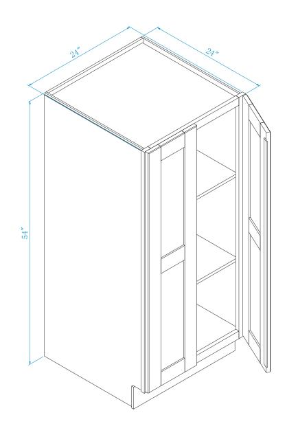
NOTE: No center stile. Batten is attached to door panel in lieu of a center stile.
