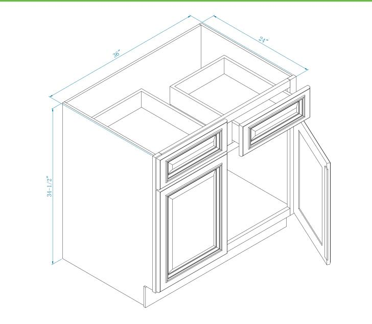
NOTE: No center stile. Batten is attached to door panel in lieu of a center stile.
