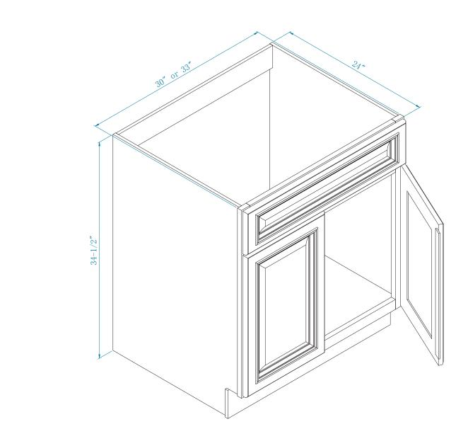
NOTE: No center stile. Batten is attached to door panel in lieu of a center stile.
