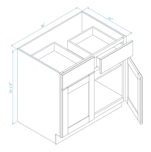
NOTE: No center stile. Batten is attached to door panel in lieu of a center stile.
