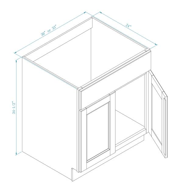
NOTE: No center stile. Batten is attached to door panel in lieu of a center stile.
