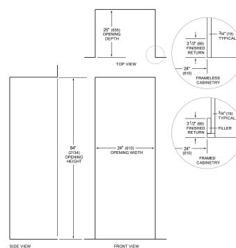
NOTE: 3<sup>1</sup>/2" (89) finished returns will be visible and should be finished to match cabinetry
