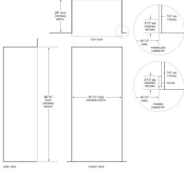
NOTE:  $3^{1/2}$ \*(89) finished returns will be visible and should be finished to match cabinetry Shaded line represents profile of unit.
