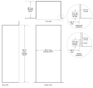
NOTE:  $3^{1/2^{\alpha}}(89)$  finished returns will be visible and should be finished to match cabinetry Shaded line represents profile of unit.
