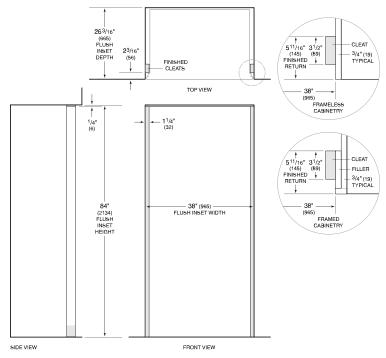
NOTE: 31/2" (89) finished returns and shaded areas will be visible and should be finished to match cabinete.
