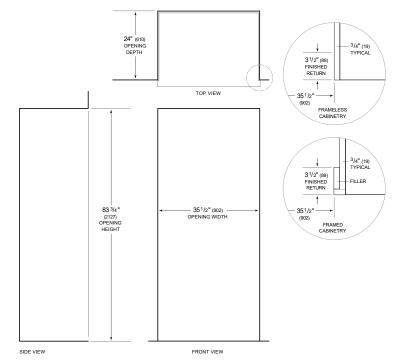
$NOTE: 3^{1/2^{\ast}}(89)$  finished returns will be visible and should be finished to match cabinetry Shaded line represents profile of unit.
