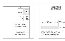
PANEL SPECIFICATIONS For complete panels specifications including width/height, weight requirements, thickness requirements and offset details visit <u>subzero-wolf.com/builtinconfigurator</u>.
